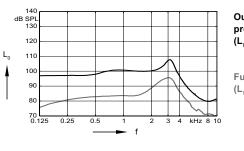
Output sound pressure level (L<sub>1</sub> = 90 dB)
